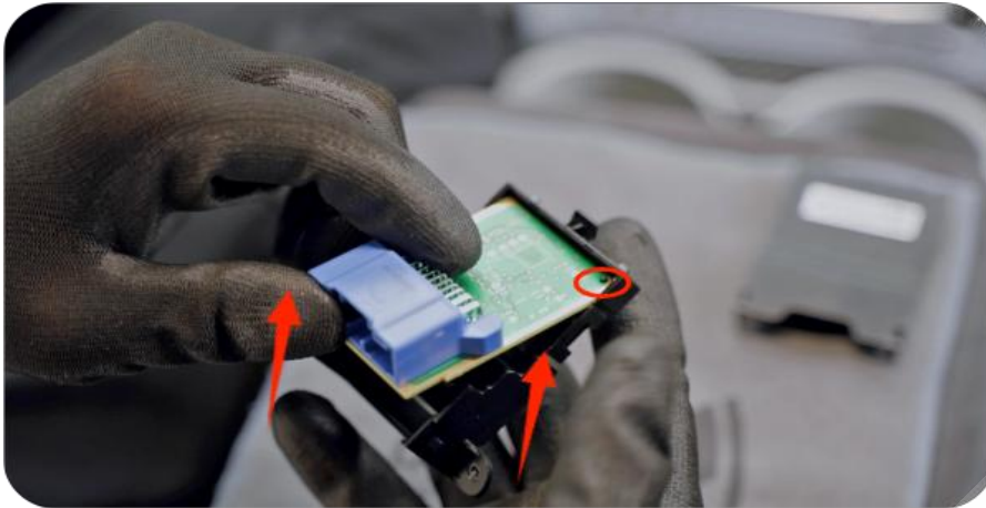
17. Take the electronic board up (note the dowel pins)
