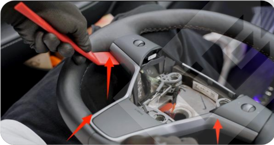
11. Pry off the middle trim of the steering wheel with the warping board
