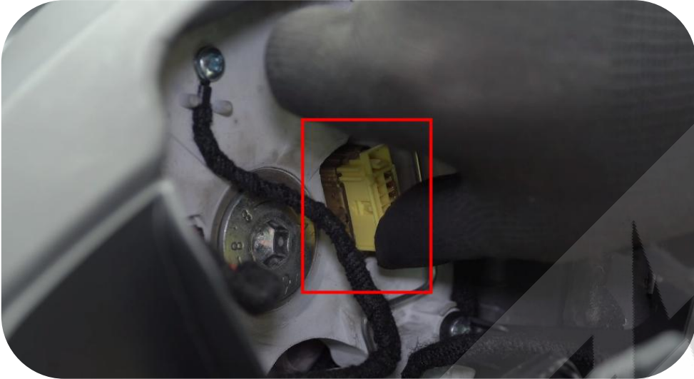
29. Insert the airbag plug into the steering wheel
