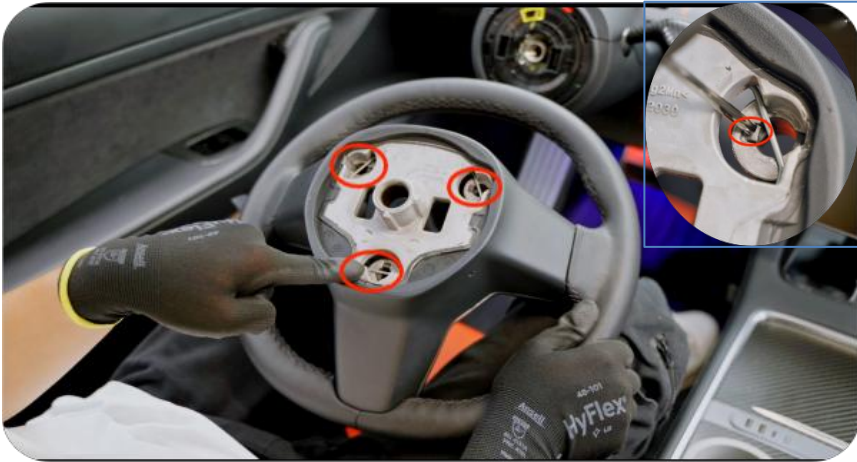
9. Use a flat-head screwdriver to pry open all 6 clip positions
