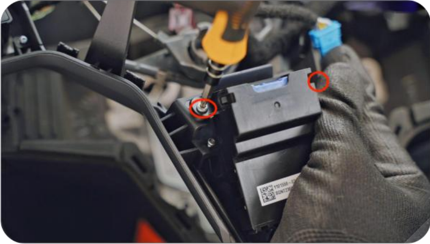
13. Remove the control box after unscrewing the 2 fixing screws with a T10 screwdriver
