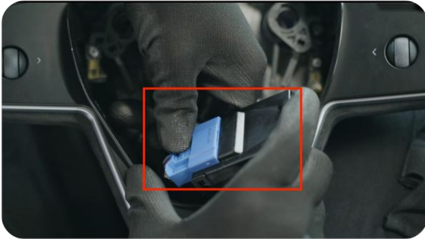
21. Insert the blue plug into the newly replaced control box
