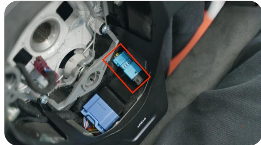
24, the heating plug is plugged next to the control box
