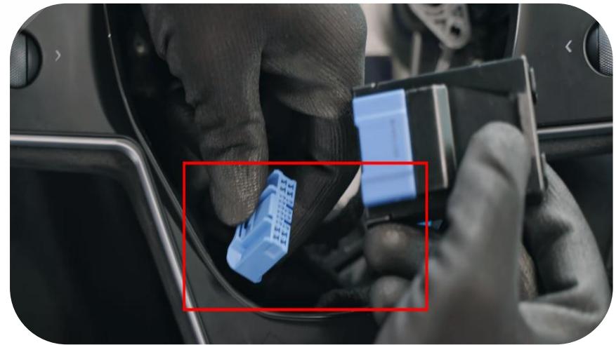
20. Find the harness plug under the steering wheel of the new CyberPack
