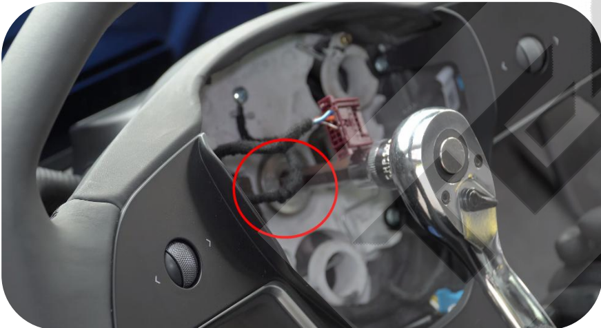
27. Use the H10 sleeve and adjustable wrench to tighten the set screws clockwise (one person can hold the sides of the steering wheel with their knees)
