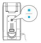
Blue light flashing (Charging) Blue light (Fully Charged)
