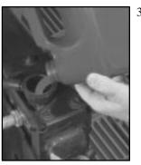
3. Fill the radiator with the proper DEX-COOL® coolant mixture, up to the base of the filler neck. (See "Engine Coolant" in the Index for more information about the proper coolant mixture.)
