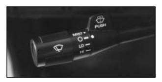
The windshield wipers are controlled by turning the band with the wiper symbol on it.
