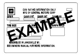
This is called the Gross Vehicle Weight Rating (GVWR). The GVWR includes the weight of the vehicle, all occupants, fuel and cargo.
