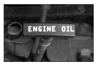
The engine oil dipstick is located on the passenger's side of the engine compartment.
