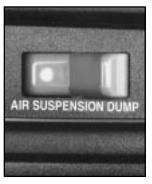
The switch to deflate and inflate the air suspension is located on the upper left side of the instrument panel above the driver's side vent.
