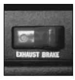
The switch is located on the upper right side of the instrument panel and turns the exhaust brake on and off.
