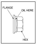
5. Oil the surfaces between the nuts and washers as shown. Do not oil the studs or the threads of the nut.
