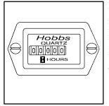
If your vehicle has this gage, it will be to the lower left of the steering column, mounted on a bracket either above or below the fuse block. It shows the total engine operating time.
