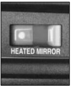
If your vehicle has heated mirrors, you'll find this switch on the upper right side of your instrument panel area, just above the radio. Use it to operate your mirror heaters to defrost or defog your mirrors.
