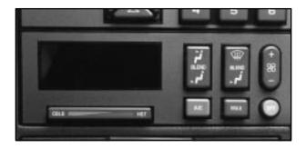
Your system has a lighted display showing each system when it is operating. During normal operation, all the lights won't come on at the same time. Only the ones displaying the current settings will light.
