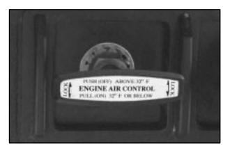
If your vehicle has this control, the handle is located on the instrument panel just to the right of the steering wheel. The control is activated by pulling the handle out and turning slightly in either direction to lock it. When the handle is pulled out, the engine air intake supply is closed off from the front scoop and an under hood air supply is opened. This control is intended only for use in cold weather (32° F (0° C) or below) where snow and ice might plug the external intake.
