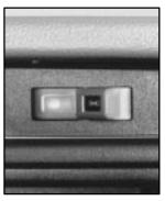
Your vehicle will have this switch only if it is designed to pull a trailer. If it has this switch, you'll find it located on the upper right side of your instrument panel, just above the radio.
