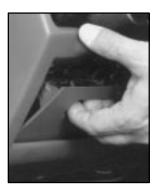
To open, pull up and out on the recessed door handle and the door will snap out. To reinstall the door, place the lower door into the bottom retainer and push the top of the door in until it snaps into place.
