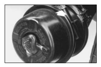
Remove the release stud and nut from the side of the brake chamber. Some chambers have studs which are visible at all times.
