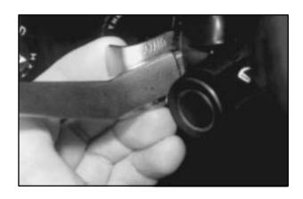
To make it work, pull out on the hazard lever until it locks into place. It works no matter what position your key is in, and even if the key isn't in.
