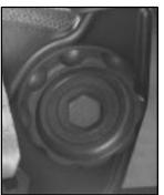
To tilt the seatback, turn the backrest tilt knob. The knob is located on the lower cushion, on the outboard side of the driver's seat and the inboard side of the passenger's seat.
