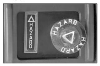
With some options, such as U86-trailer wiring or RQ3-tractor application, you will have this switch. This switch replaces the hazard switch mounted on the steering column. It is mounted in the instrument panel, usually to the left of and below the steering column.
