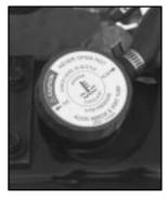
The radiator pressure cap must be tightly installed with the arrows on the cap lined up with the top of the overflow tube. This will prevent coolant loss and possible engine damage from overheating.
