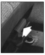
To adjust the height of the cushion, lift the cushion height adjustment handle up and forward. You can choose between two settings. The handle is located underneath the seat, in the front.
