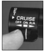
If your vehicle has this feature, it is located at the end of the turn signal/multifunction lever.
