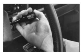
This feature lets you apply the trailer brakes without applying the tractor brakes. You can apply the trailer brakes a little or apply them all the way if you have to. Use this control only when you're driving. Don't use it for parking or to hold the rig on a hill.
