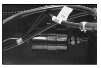
If your vehicle is equipped with the optional Davco spin-on type filter, it is also located in the component box.
