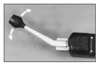
To signal a turn, move the lever all the way up or down. When the turn is completed, move the lever back to the center position.
