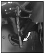
To release the parking brake, first push down the regular brake pedal. Then, push the parking brake lever all the way down and shift the automatic transmission to NEUTRAL (N).
