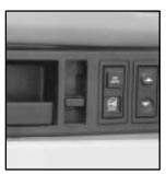
Push the switch marked LOCK to lock both doors at once.
