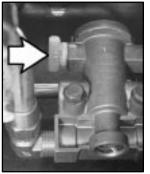
To turn it on in cold weather, turn the valve so that the word ON is on top. When the temperature is above freezing, turn the valve to OFF. Use only methyl alcohol in this system.
