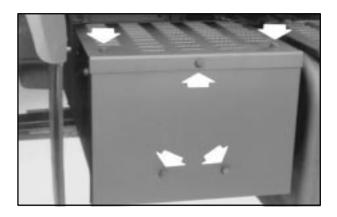
To get into the box, you first have to remove the top cover. To do that, remove the two 8 mm bolts on top and the single 8 mm bolt at the top front. Then, pull the cover toward you and lift it off.
