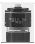
When the CHANGE FILTER indicator appears in the sight glass, it's time to service the air filter. After the air filter is properly serviced, the indicator can be reset by pushing the button on top of the indicator to reset it.
