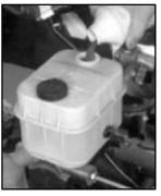
If it's low, add enough fluid to fill the reservoir to the proper level.
