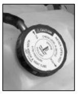
The surge tank pressure cap must be tightly installed with the arrows on the cap lined up with the top tube of the coolant surge tank.
