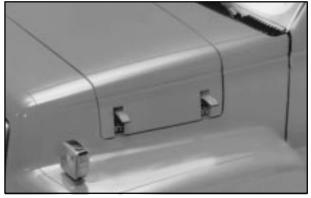
If your vehicle has the optional hood access panels, you can easily get to one side of the engine or the other as you need to.
