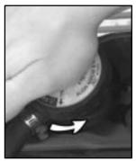
2. Then keep turning the pressure cap, but now push down as you turn it. Remove the pressure cap.
