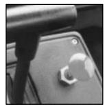
The switch for the rear axle shift control is on the shift tower to the right of the shift lever.
