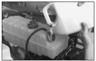
3. Then fill the coolant surge tank with the proper coolant mixture, up to the COLD FULL mark.
