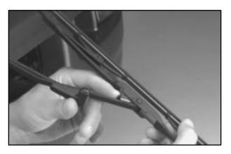
Windshield wiper blades should be inspected at least twice a year for wear or cracking. See "Wiper Blade Check" in Section 7 of this manual under Part B: "Owner Checks and Services" for more information.
