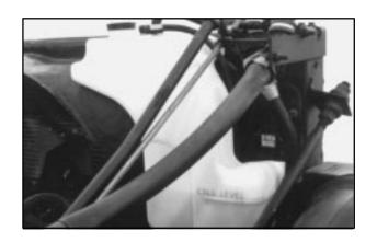
Coolant Recovery Tank (Gasoline Engines -- Sloped Hood)
