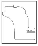
When the engine is cold, the coolant level should be above the HOT LEVEL mark on the vehicle with the specialty hood, or at or above the COLD LEVEL mark on the vehicle with the sloped hood.
