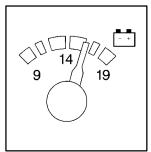
When your engine is running, the voltmeter gage, at the lower left of the instrument panel cluster, shows the charging system voltage.
