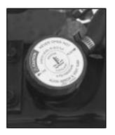
8. Then reinstall the pressure cap. At any time during this procedure if coolant begins to flow out of the filler neck, reinstall the pressure cap. Be sure the arrows on the pressure cap line up like this.
