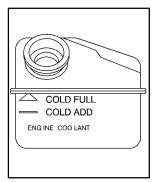
The coolant level should be at COLD ADD or higher. If it isn't, you may have a leak in the radiator hoses, heater hoses, radiator, water pump or somewhere else in the cooling system.
