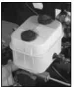
If your vehicle has hydraulic brakes, there's a brake master cylinder. The brake master cylinder reservoir is here. Refer to the Maintenance Schedule to determine when to check your brake fluid.
