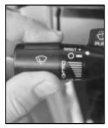
You can set the wiper speed for a long or short delay between wipes. This can be very useful in light rain or snow. Turn the band to choose the delay time. The closer to LO, the shorter the delay.
