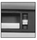
To lock your door from the inside, slide the manual lock control down.
