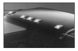
Your headlamps switch will not operate these lamps. You can use the switch to manually blink the marker and clearance lamps by simply turning it on and off.
