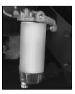
If you have a Caterpillar<sup>®</sup> diesel engine, you may have this spin-on filter. It is located in the component box on the driver's side behind the fender.
