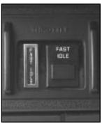
The manual fast idle switch is located on the lower portion of the instrument panel just to the left of the steering wheel.
