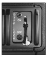
If your vehicle has this feature, the control is located at the lower right corner of the instrument panel.
