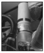
If you have a Caterpillar<sup>®</sup> diesel engine, you may have this spin-on filter and fuel separator/heater. It is mounted on the driver's side of the engine.
