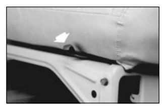
If your vehicle has a bucket or bench seat, you can adjust it with this lever located at the front of the seat.
