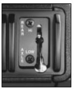
The lever for the rear axle shift control is either at the lower right corner of the instrument panel or on the shift lever.
