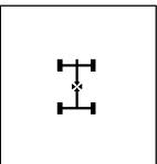
This light located on the instrument panel cluster is on when the inter-axle differential lock system is in use.
