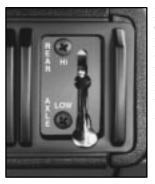
If your vehicle has a Controlled Traction or Locking Differential axle, the control is located at the lower right corner of the instrument panel. You'll see this control on single rear axle vehicles. If you're approaching a slippery surface where it looks like one or even both wheels may start to slip, you can use this control. It locks your rear differential so that power is transmitted equally to both rear wheels.
