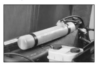
Coolant Recovery Tank (Gasoline Engines -- Specialty Hood)
