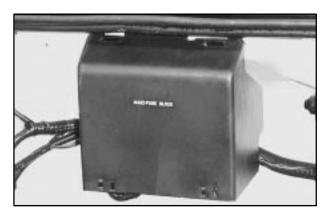
To access the maxi-fuse block, gently squeeze both sides of the cover to unlatch the tabs at the top. Then, unsnap both attachments at the bottom and remove the cover.
