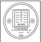
This optional gage is in the lower center of the instrument panel cluster. It monitors the engine air filter.
