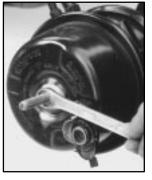
Using a wrench, turn the stud nut clockwise several turns to release the brakes. Follow the same procedure to release the other brake.
