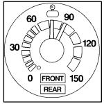
If your vehicle has air brakes, this gage at the center of your instrument panel cluster shows the air pressure for both your front and rear brake systems.
