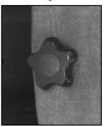
To get more support in the lumbar area of your back, turn the lumbar adjustment knob. The knob is located on the upper cushion, on the inboard side of the driver's seat and the outboard side of the passenger's seat.
