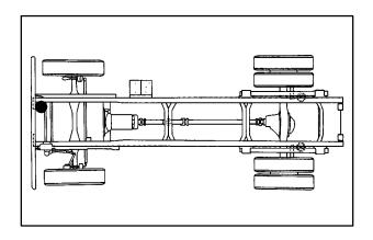
The alcohol injector helps prevent moisture in the air brake system from freezing. Use it only in cold weather, 32°F (0°C) or below.
