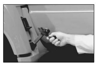
To tilt the hood forward, pull out on each of the hood latches. If the hood is equipped with hood access panels, make sure the panel latches are locked down before lifting the hood open.
