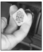
If your vehicle has air brakes, you will have this control. Pulling it out applies the parking brake. The PARK BRAKE light will come on when the air parking brake is applied.
