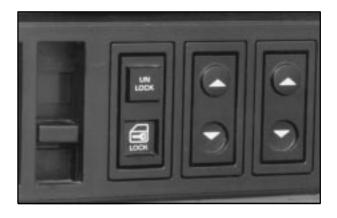
Push the switch marked with an up arrow to raise the window. Push the switch marked with a down arrow to lower the window.
