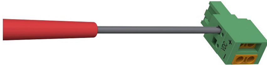
FIGURE 7-3. Opening the power connector terminals
