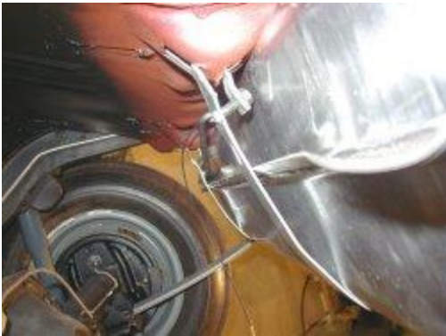
Closeup of sheet metal screws through strap at rear strap mount position.
