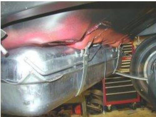
Step 6. Pull the strap up into place and insert the retaining bolts. Secure with nuts provided in Quanta Products kit STB-1.
