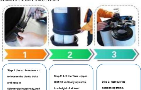
gently tap the clamp with a rubber mallet to loosen it.
