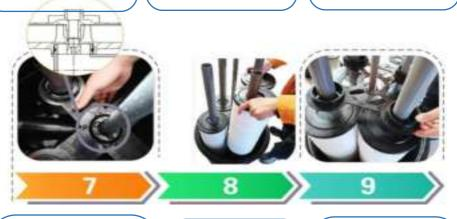
Step 7: Check if the positioning lower seat is detached. If it is,apply lubricant to the O-ring of the inner-threaded elbow pipe. Then align the four fixing holes of the position- ing lower seat with the support columns of the barrel body and press them in.
