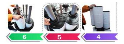
Step 6: Lift the four lower filters vertically upwards to a height of at least 95cm before removing them.
