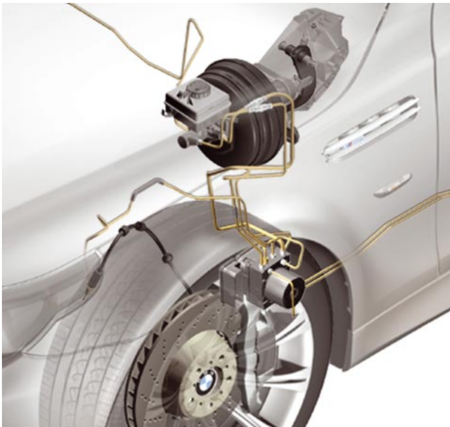
Mounting Location of DSC Control Unit and Hydraulic Unit
