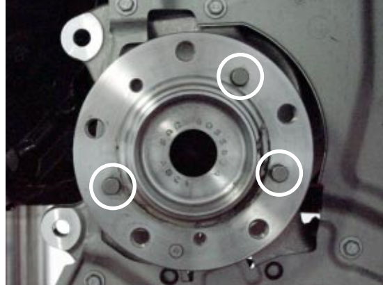
Detail of Rotor Alignment Pins on Hub
