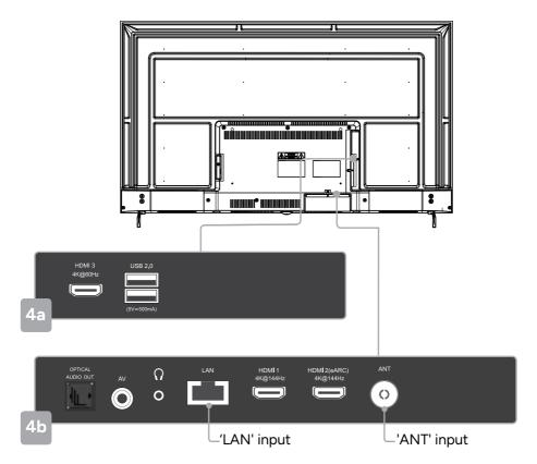
Following these options, the **Auto Tuning** screen will appear. Ensure you have an antenna cable connected to the 'ANT' input port at the back of the TV **(4b)**.
