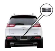
**Electronic Liftgate Release/Liftgate Passive Entry Location**
