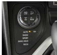
2-Speed 4x4 Switch (with Rear Lock)
