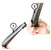
Wiper Blade Removed From Wiper Arm
