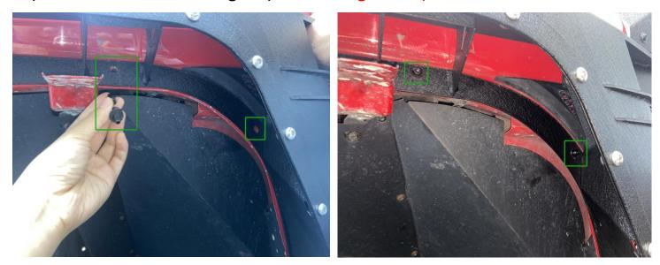
Step 6: Finally, when installing the rightmost hole, use the extended rod tool to screw in the screw, and then cover the plug back.
