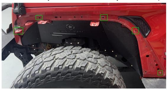
Step 2: Before installation, please apply rubber strips along the edges of the fender (green line) to prevent scratching the car surface.
