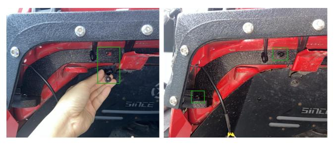
Step 5: And then install the middle two holes. Use the Button Head Socket Cap Bolts Screws (M6\*20) groups. Don't tighten up those bolts.
