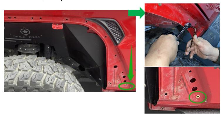
Step 4: Next, Lift up the front fender flare and install the left two holes. Use the Button Head Socket Cap Bolts Screws (M8\*20) groups and Button Head Socket Cap Bolts Screws (M6\*20) groups. Don't tighten up those bolts.
