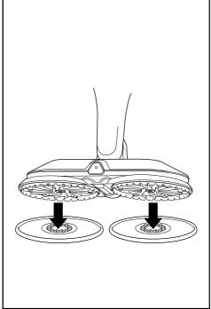
Insert the Mop Handle into the Steam Mop Body 2. To attach the Dirt Grip Soft Scrub Pads, place **BOTH** pads flat on the floor with plastic rings facing up. Align the unit directly over the plastic rings on the pads. Gently lower the Mop **Head** onto the pads, pressing until the pads are secure.
