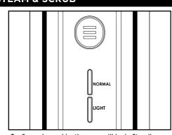
2. Once plugged in, the mop will be in Standby mode and both steam setting lights will blink. Press the Mode Button to select Light or Normal mode, then wait 20 seconds to allow steam to release.
