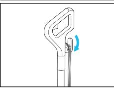
Twist the quick-release cord holder to unwrap the power cord completely. Plug into an electrical outlet.
