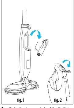
Unplug the steam mop before filling the Water Tank. To remove the tank, pull it out, away from the mop tank (fig. 1). Pull the top rubber fill cap back and fill the tank with cold or room temperature water ONLY (fig. 2).
