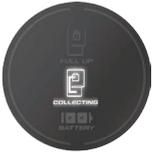
The "COLLECTING" sign will be high brightness while the collector is working.
