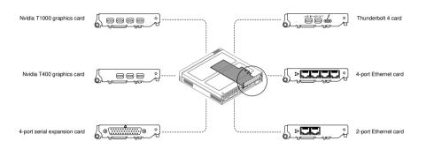
You can configure the expansion module to support many types of devices and scenarios, including but not limited to the following:
