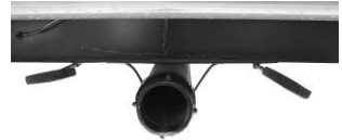
Black/Grey Tank Drain and Valves
