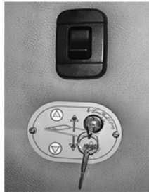
Fig.2 Key OFF (Vertical)
