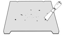
② The residue of the platform filaments can be scraped off with a blade. Be cautious of safety when using.
