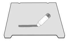
③ When the first layer of the model is not glued, it is recommended to apply glue stick evenly on the surface of the platform.
