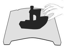
① Together with the flexible platform after the printed model has been cooled down Remove from the device and partially bend the platform slightly to separate the model from the platform.(No excessive bending of the platform to prevent it from being deformed and unusable)
