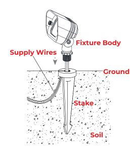
Pass supply wires through the center hole of the stake and thread the stem onto the stake. Hand tighten until snug. Clear away an area in the ground and lay supply wires into wireway slots.
