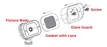
Unlock the screws to remove the glare guard and gasket with lens from the fixture body.
