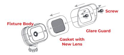
Place the gasket with new lens, the glare guard back onto the fixture body and secure with previously removed screws. Hand tighten until snug.
