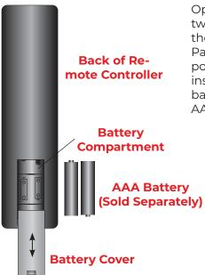
Open the battery cover, install two AAA 1.5V batteries into the battery compartment. Pay attention to the "+"/"-" polarities of the battery when installing. Always reinstall the battery cover after installing AAA 1.5V batteries.
