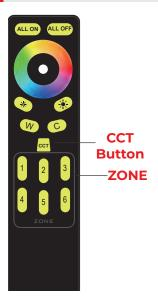
The preset color temperatures of the CCT button are 2200K, 27000K. 3000K and 4000K.
