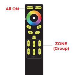
1. To control lights by group, Select the lights by pressing the zone they are in. And then press respective function buttons to adjust the lights.
