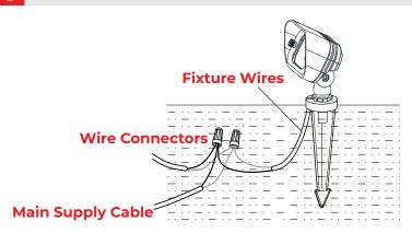
Strip two leads from fixture wires. Using two UL listed wire connectors (not provided), connect leads from fixture wires to main supply cable leads.
