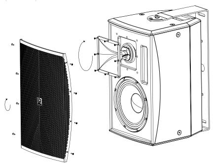
To rotate the VEXO1xx's horn, the grille must be removed first. To do this, the eight screws on the sides must be unscrewed.
