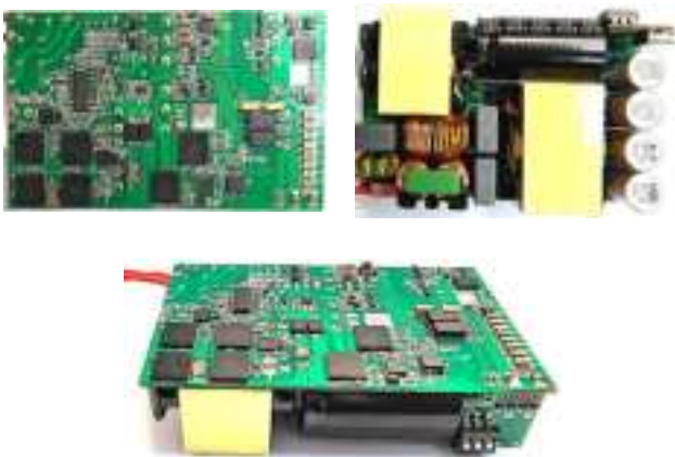
Figure 6: EVB of 240W TPFC + 2SW QR Flyback
