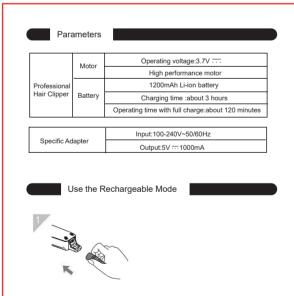
1 . Insert the charger into the tail of clipper , connect to the
