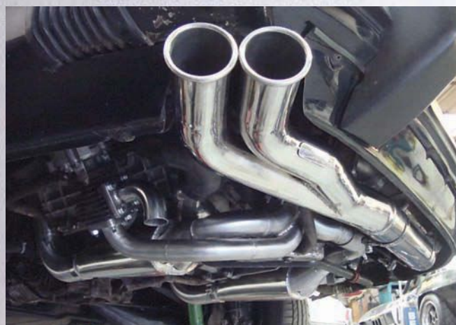
Porsche 3.3 complete system - standard style tailpipes
