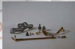
Original RS/RSR Oil Cooling system
