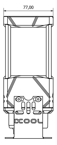
General tolerance: ± 0,25mm Dimension in millimeter
