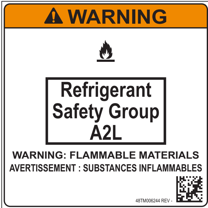
Fig. 63 — A2L Refrigerant Safety Group Warning Label
