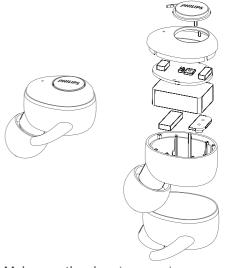
Make sure the charging case is disconnected from the USB charging cable before removing the battery.
