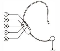
1. Power switch: power on and power off 2.M mode key: unlock, frequency conversion, frequency interruption, frequency binding 3. Volume key: volume up
