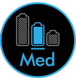
The screen shows the machine set to Med mode with a blue battery showing that this will give a medium length of battery life.
