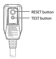
The circuit breaker should be tested periodically by pressing the **TEST** button then the **RESET** button. If the **TEST** button does not cause the circuit breaker to trip, or if the **RESET** button will not stay engaged, unplug the air conditioner immediately and contact an Insignia technician.
