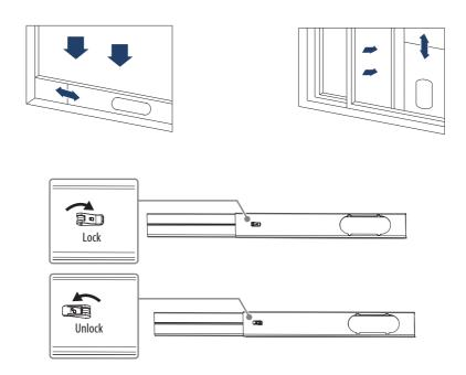
4 Insert the hose adapter into the vent panel, then slide the adapter until it clicks into place.
