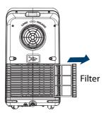
2 Clean the filter with a vacuum cleaner. If the filter is very dirty, it can be washed by hand in warm water with a mild detergent.
