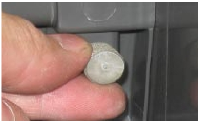
Remove Thumb Screw Holding Curtain
