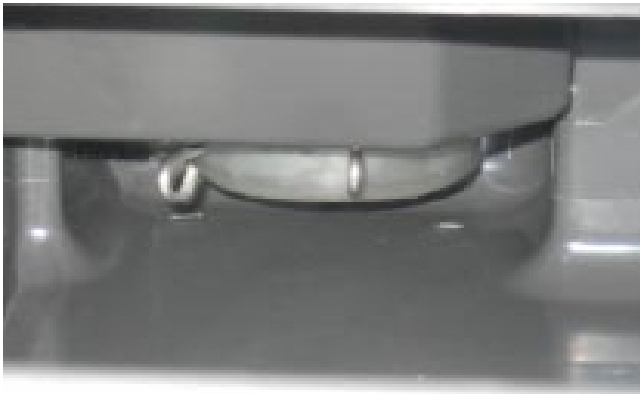
Remove Drain Cap
