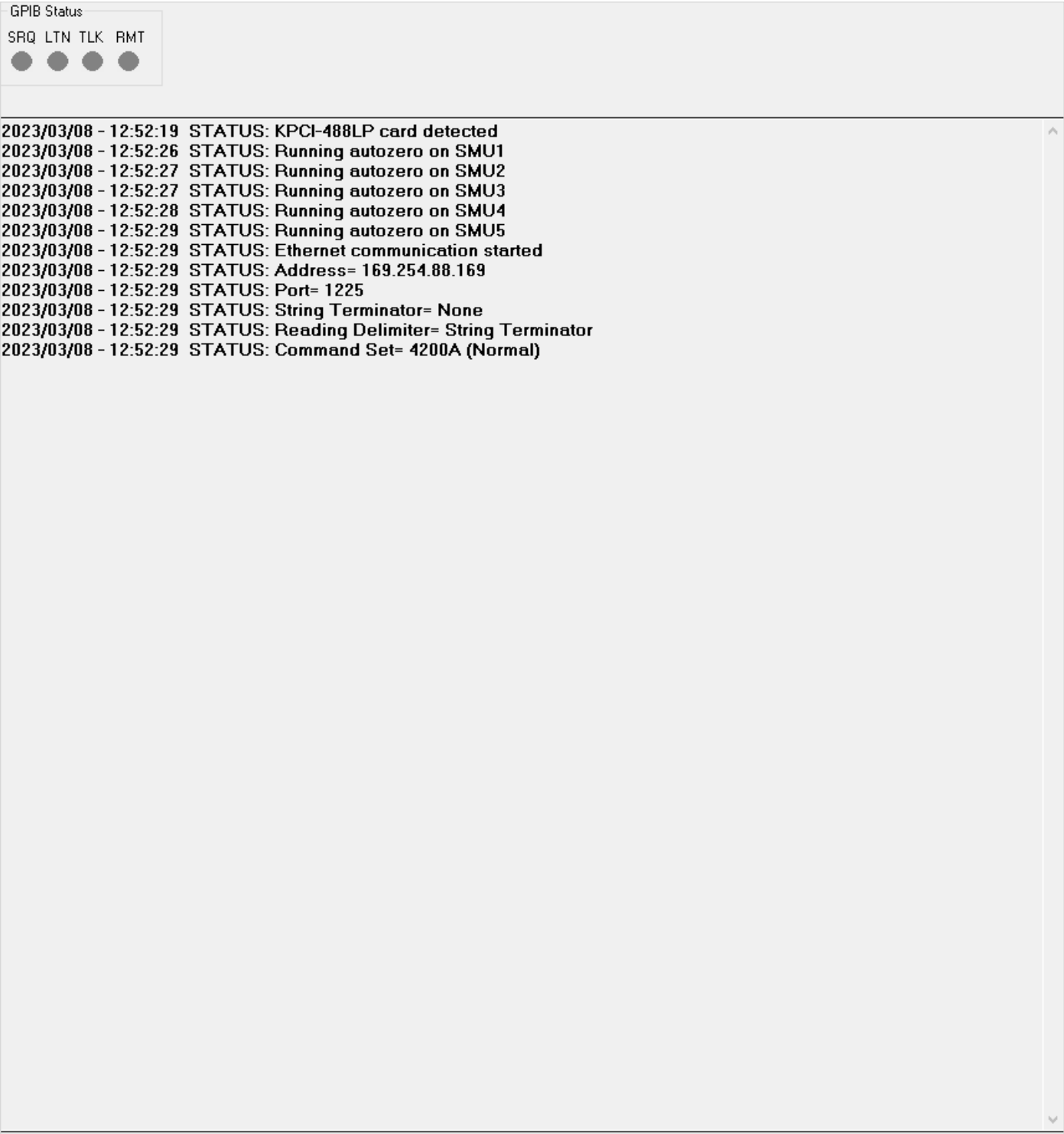
Figure 6. KXCI interface connected with ethernet.
