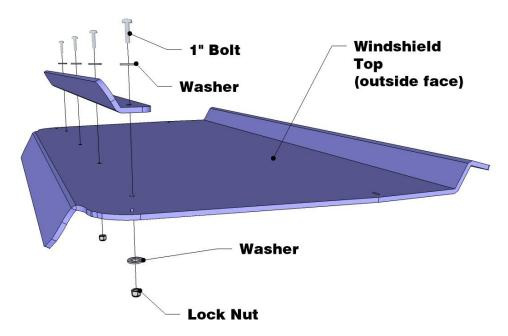
5. Now you are ready to place the windshield on the Bobcat and attach to the roll cage. NOTE: THE BEND AT THE TOP OF THE WINDSHIELD SHOULD GO BELOW THE TOP TUBE. The diagram
