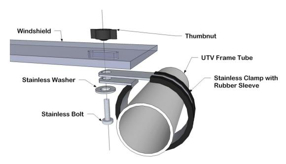
6. Now Place the two halves onto the frame as shown on the next page. (diagram not Bobcat)
