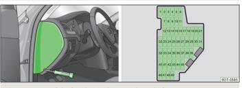
Fig. 198 Cover of the fuse box in the control panel / fuses
