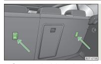
Fig. 158 Anchor evelets on the TOP **TETHER system**
