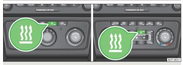
Fig. 109 Button for switching on/off the system directly on the operating part of the air conditioning/Climatronic
