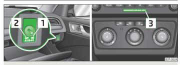
Fig. 154 Key switch for front passenger airbag/warning light for front passenger airbag activation/deactivation
