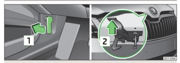
Fig. 161 Bonnet release lever/release lever
