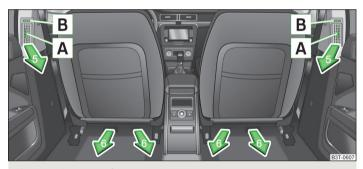
Fig. 106 Air vents at the rear
