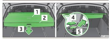
Fig. 87 Foldable luggage compartment cover: pull out and roll up / take out
