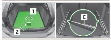
Fig. 95 Boot: partially pulling out the variable loading floor
