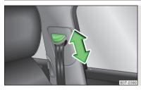
Fig. 148 Front seat: Seat belt height adjuster
