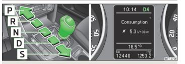
Fig. 123 Selector lever / display
