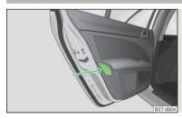
Fig. 76 Left rear door: Stowage compartment for an umbrella
