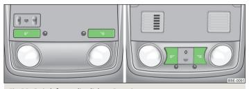
Fig. 36 **Switch for reading lights - 2 versions**
