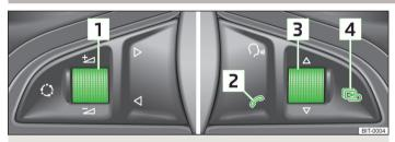
Fig. 111 Multifunction steering wheel: Control buttons for the telephone
