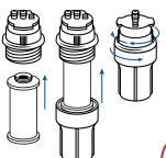
Press new replacement filter to the top of the filter housing using the appropriate color coded filters. Then, reconnect the bottom of the filter housing to the top half. Ensure connection points are correctly aligned, then turn clockwise to tighten. Continue this step for the second and third filter housing.
