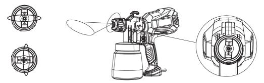
7) Turn on the power switch and press the trigger to spray paint.
