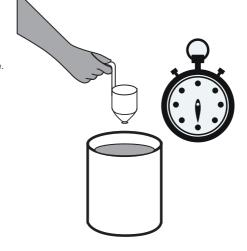
DIN-S: The time for the liquid to run out of a funnel.
