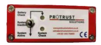
The Control Box can test the continuity of the wiring, switches and firing mechanism. The switch used is a 3 way switch and any testing should be carried out with the switch in the middle position.
