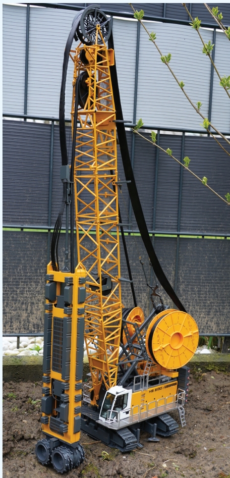
Equipped with the impressive slurry wall cutter.
