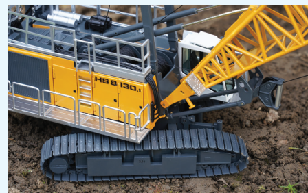
Additional undercarriage counterweight and fairlead for dragline operation.
