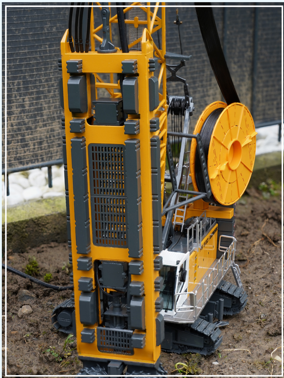
Massive slurry wall cutter with wheels, rotating device and flaps.
