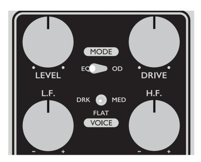
**MODE SWITCH:** This switch selects between two different gain levels, with subtle voicing tweaks designed to get the best out of each mode.
