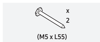
Screw for mounting on wall (6011-008215)
