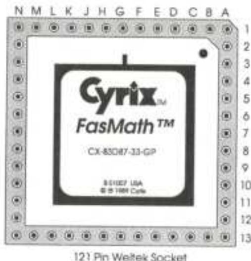
Figure 3(b). Completed installation in 121 Pin Socket.
