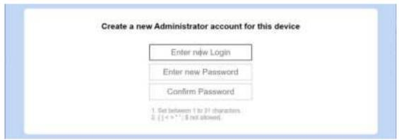
NOTE: For older firmware versions, the default user name is "admin" and the default password is the last 6 characters of the MSNSwitch's MAC address (upper case). See the bottom label for the MAC address.
