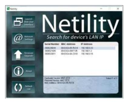
The **Network Settings** button allows you to configure the IP address and related network parameters of the MSNSwitch as well as set the password. The **Launch Web User** Interface will open the MSNSwitch's internal web server in your default browser.
