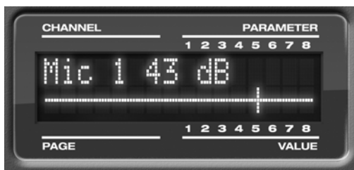
Figure 4-3: The LCD gives you feedback as you turn the TRIM knobs for the four mic/guitar inputs.
