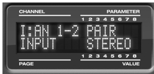
Figure 4-5: The settings for analog inputs 1 and 2 (as a pair).
