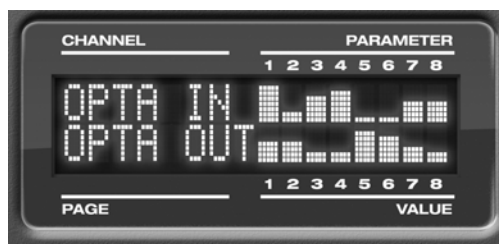
Figure 6-4: Multi-channel metering in the LCD.
