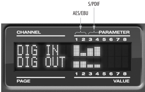
Figure 6-5: Viewing AES/EBU and S/PDIF level meters in the LCD.
