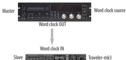
Figure 4-21: Slaving the Traveler-mk3 to word clock. For the Traveler-mk3 clock source, choose 'Word Clock In'.
