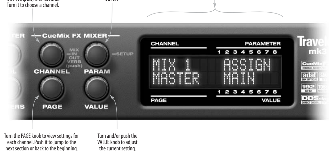
Figure 6-10: The Traveler-mk3 front panel LCD controls.
