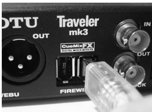
Figure 4-1: Connecting the Traveler-mk3 to the computer.
