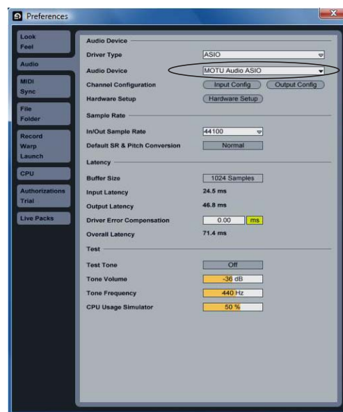
Figure 7-3: Enabling the Traveler-mk3 in Live.
