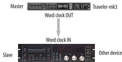
Figure 4-20: Slaving another digital audio device to the Traveler-mk3 via word clock. For the Traveler-mk3 clock source, choose any source besides word clock, as it is not advisable to chain word clock.
