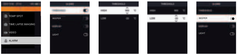
Figure 12.5 Configuring the high and low alarms.
