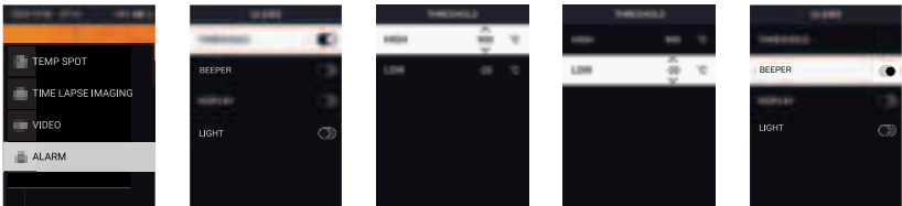
Figure 11.16 Configuring the high and low alarms.
