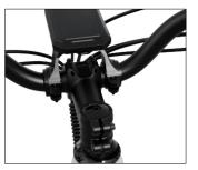
Cover the stem screw with Steam screw plugs for protection.
