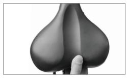
3 Adujst the seat and the head of the seat is parallel with the top tube.
