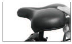
Move the seat up and down by sliding the seatpost in or out of the seat tube.
