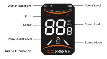
SPEED MODE: Average speed (AVG SPEED), maximum speed (MAX SPEED), real-time speed (RT
