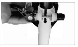
Open the quick-release lever by swinging the lever open and outward fully.
