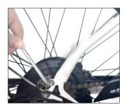
Loosen the four screws in 2 the seat stay.
