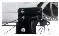
Make sure the kickstand is align with the two holes in the frame.
