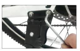
Tighten the screws to fix the kickstand in place.
