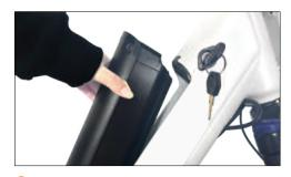
3 Prop up the battery with your left hand and then remove the battery with both hands.
