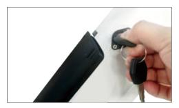
1 Put the key into the lock, turn it to the left which is the direction for unlocking.
