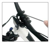
After making sure the 5 Tighten the screws to fix 6 the handlebar in place.
