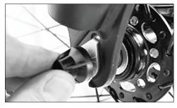
3 Tighten the nut onto the fork.
