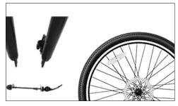
1 Locate the quick-release lever. Open the lever and remove the thumb nut, safety hook, cone spring (opposite the lever). Keeping the washer and other safety hook and cone spring in place on the lever side.
