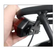
4 Assembly the taillight into the rear rack. Screwing the nuts.
