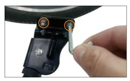
Take out the kickstand and loosen the two screws on top.
