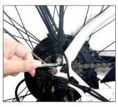
Align the rear rack with the seat stay and tighten the screws.
