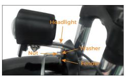
Take out the headlights and screws (including1xBolt,1xWasher, and 1xNut) Slide the fender through the fork. Reattach the bolt, washers.fender, headlight, and nut (in that order) with 5mm wrench.
