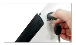
The battery can be charged off the bike. To remove the battery, turn the key to the left position (see the previous remove battery section for details).
