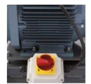
**ON/OFF isolation switch**NI versions incorporate safety switch, stop / start.
