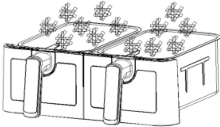
4. Slide the pan back into the Hot-air fryer and align the guides in the body of the fryer.
