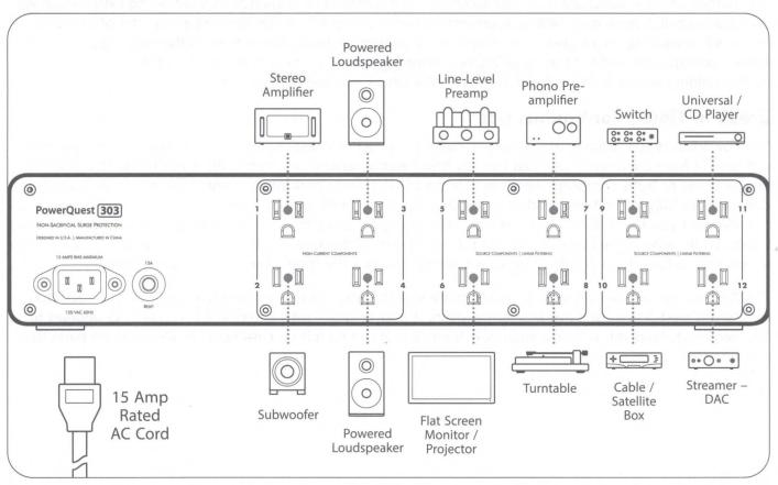
**Note:** Outlets 5 through 12 are subject to many variables and circuit conditions, so experimentation for best results is encouraged. Power amplifiers must be connected to outlets 1 through 4.
