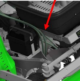
Route the hoses from the plow hitch along the right side of the hopper, up through the opening in the hopper shield, and to the control valve.
