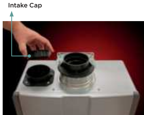
For PVC/CPVC configurations, the intake cap is removed and discarded. With this option, installers can use three- or four-inch PVC/CPVC pipe for the intake and exhaust.
