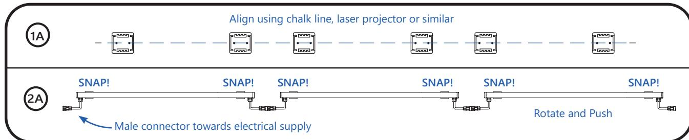
**Parallel Layout** *NOTE: the recommended maximum space between parallel luminaires is 10" (245mm) for better optical uniformity.*
