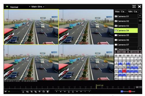
Figure 6-19 4-ch Synchronous Playback Interface
