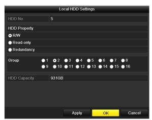
Figure 10-13 Local HDD Settings Interface
