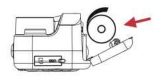
3. Before closing the paper tray, pull on the paper so that a short piece sticks out when the paper compartment door is closed.
